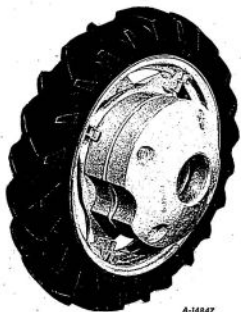
Illust. 94—First and Second Rear Wheel Weights Mounted on Wheel.
