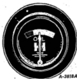
Illust. 6—Oil Pressure Indicator, Showing Needle in Correct Operating Position.
