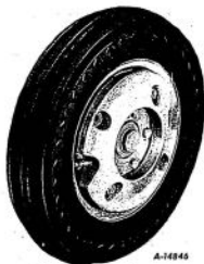
Illust. 92—First Front Wheel Weight Mounted on Wheel.
